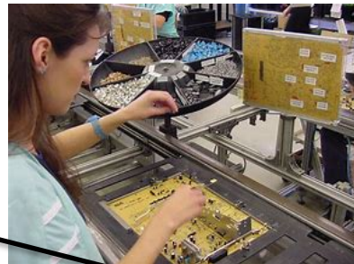
Figure 2c. ... Requiring Moving from Labor Intensive Manual Insertion and Hand Soldering ... Component Insertion and Placement Robot
