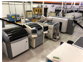
Figure 2c. ... Requiring Moving from Labor Intensive Manual Insertion and Hand Soldering ... Component Insertion and Placement Robot
